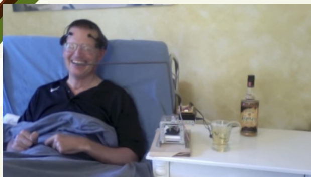
Fig. 1. Our BMI-controlled robot providing a user with a drink. The BMI consists of three components, (i) the EEG recording system, (ii) the RGB-D camera and (iii) the robotic manipulator. The EEG is used to detect go-commands from the user. The RGB-D camera detects the mouth of the user as well as the drinking cup. The robotic manipulator grasps the cup, serves the drink to the user and places the cup back to the table.
